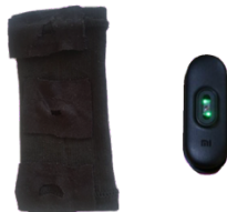
Figure 1. A Xiaomi Mi band 2 sensor (right image) with the inside of our wristband prototype capable of accommodating three of the Xiaomis using three pockets (left image).
